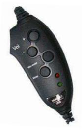
Electret Condenser Microphone -47 ± 2dB (0dB=1V/Pa, 1kHz) Low Impedance 1. Omni( ), 2. N/C ( 20-16,000 Hz 10V 2V Max. 0.4mA More than 40dB
